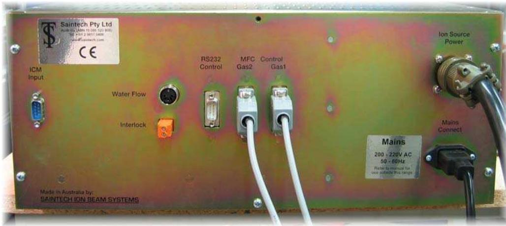
Figure shows the rear panel connections for a Dual Gas System.
