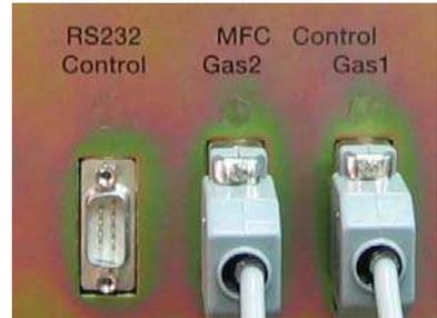
Only one (1) "MKS" brand of mass flow controller can be connected.
