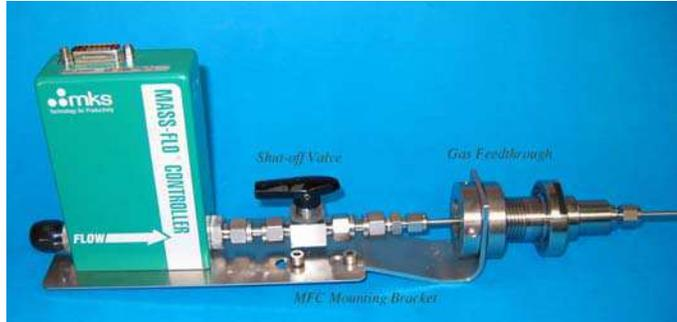
1. Install the gas feedthrough into the relevant baseplate feedthrough port and secure in place. Remove the 1/8" Swagelock nut and ferrules from the vacuum side of the fitting.
