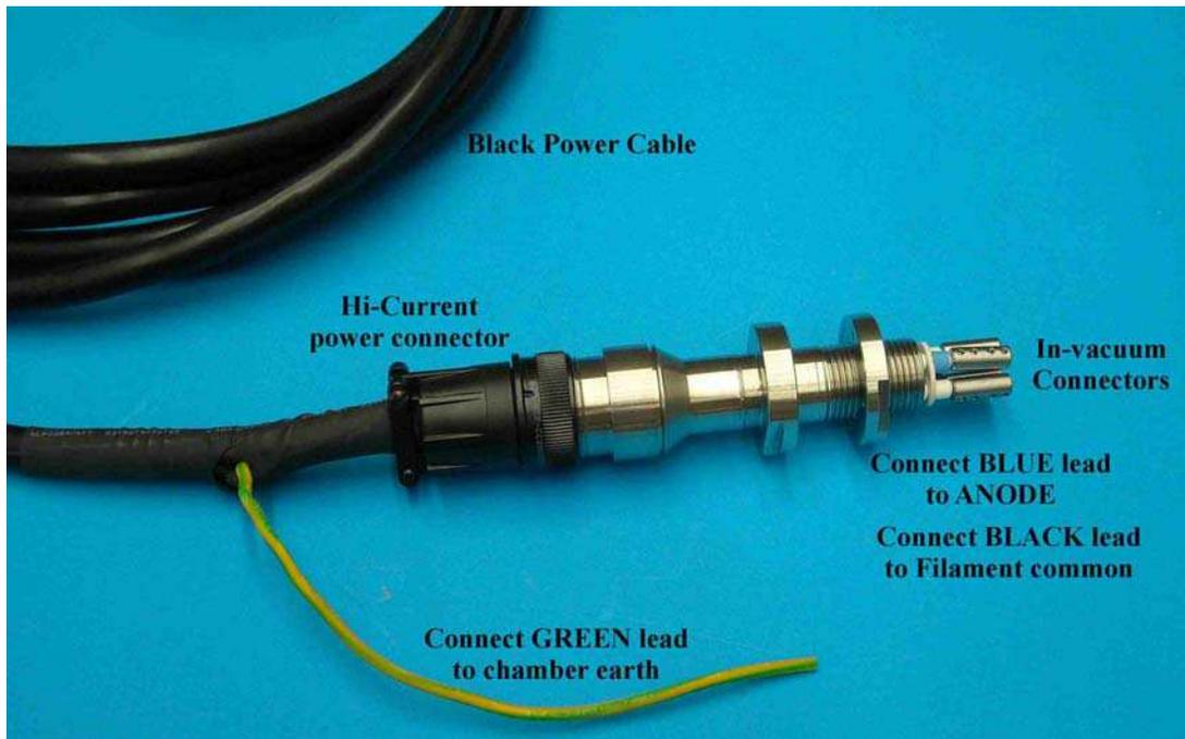
The ion beam system is supplied with an electrical feedthrough assembly to ensure ease of installation and safe and secure operation. The assembly comprises a 1" (or 32mm) standard baseplate 4-pin electrical feedthrough and a high current power connector. Figure above shows the complete assembly.
