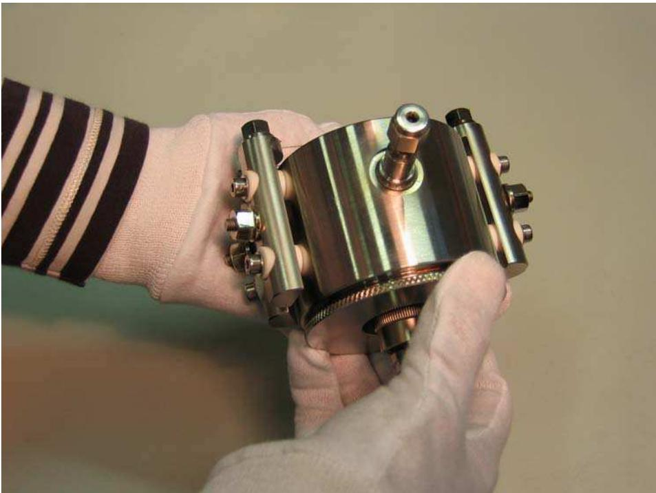
Step 2. Unscrew the knurled assembly nut from the base of the ion source
