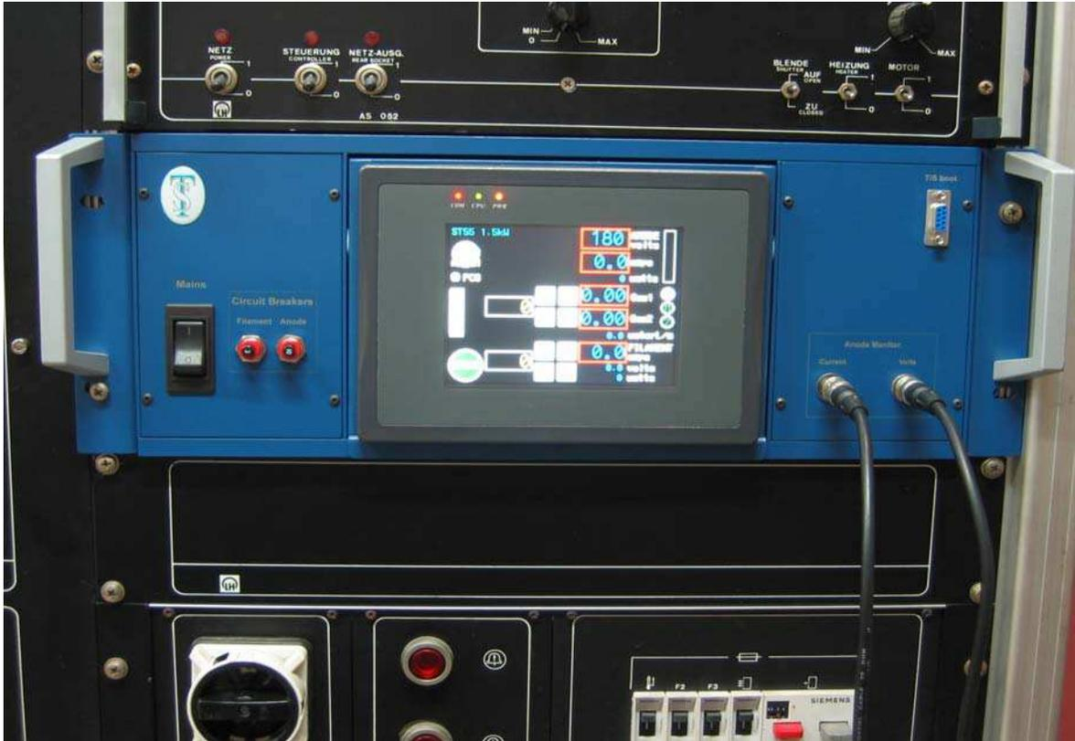
Figure above shows the power supply installed into a conventional 19" instrument rack. The tilting touch screen allows the power supply to be mounted low in the rack and still provide good visibility for convenient operation.
