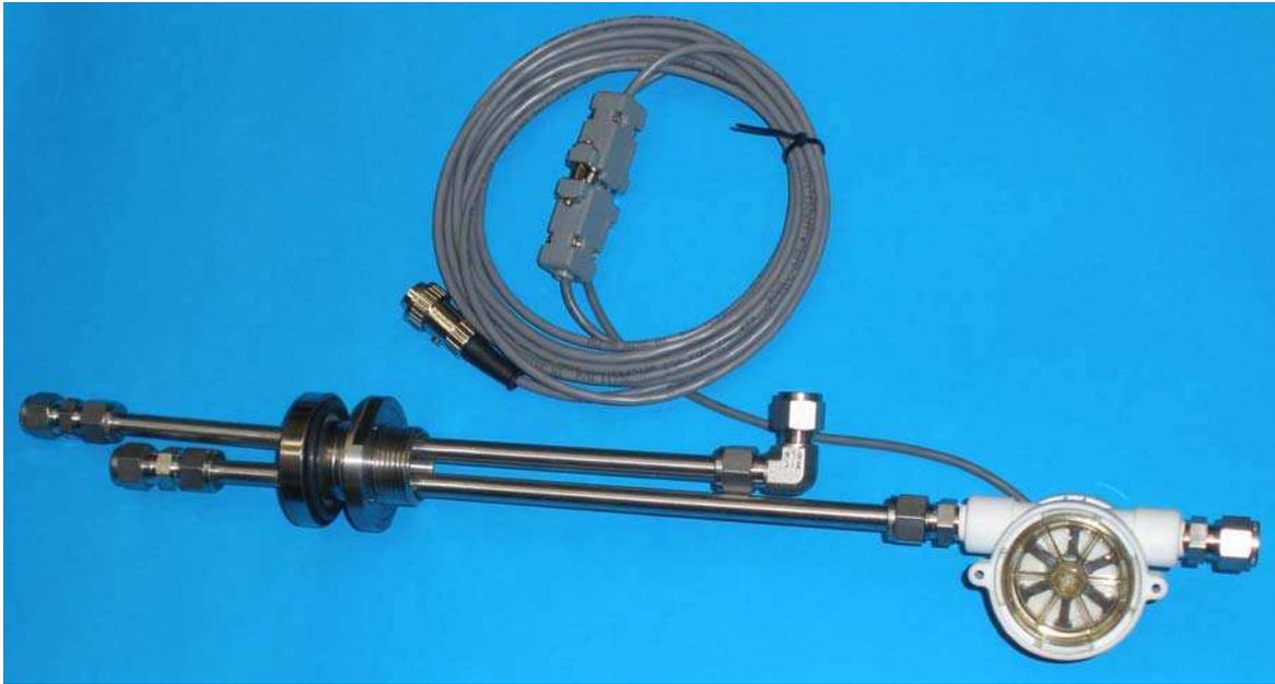
Above figure shows the water flow monitor in relative position to the vacuum feedthrough and connected using a Swagelock straight union. Note that the actual WFM shown above may be of different design or manufacture to that supplied.
