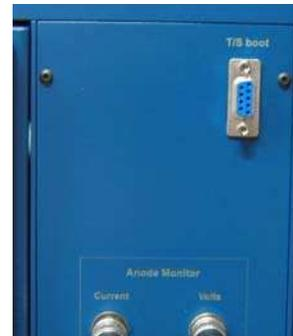
This connector is only used if the Touch Screen software is to be upgraded. It is suggested that a small length (12 inches) adapter cable be made to connect onto the remote RS232 communications cable. The ends of the adapter cable will have to be marked as to where they are connected, as both are male.
