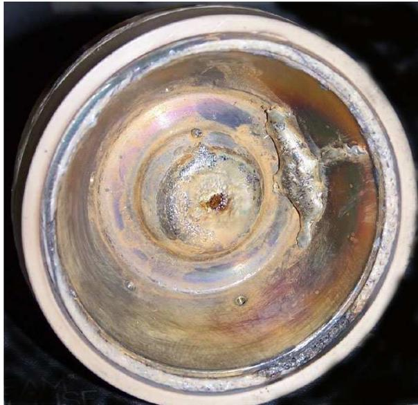
**Picture shows an ST55 anode after running the source for a few minutes without cooling water. The anode was not repairable and the rare earth magnet and anode insulator required replacement**
