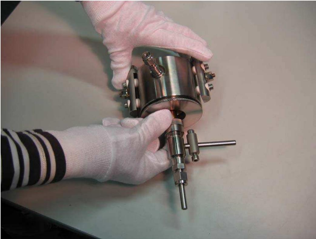
Step 1 Remove water assembly. The water manifold remains attached to anode assembly by circlip. See below for disassembly of the water manifold assembly.
