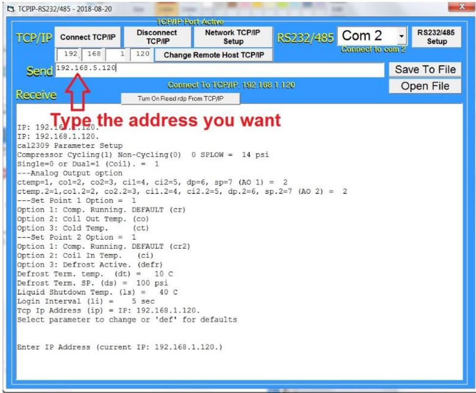
Figure 3-32, Enter new IP address
