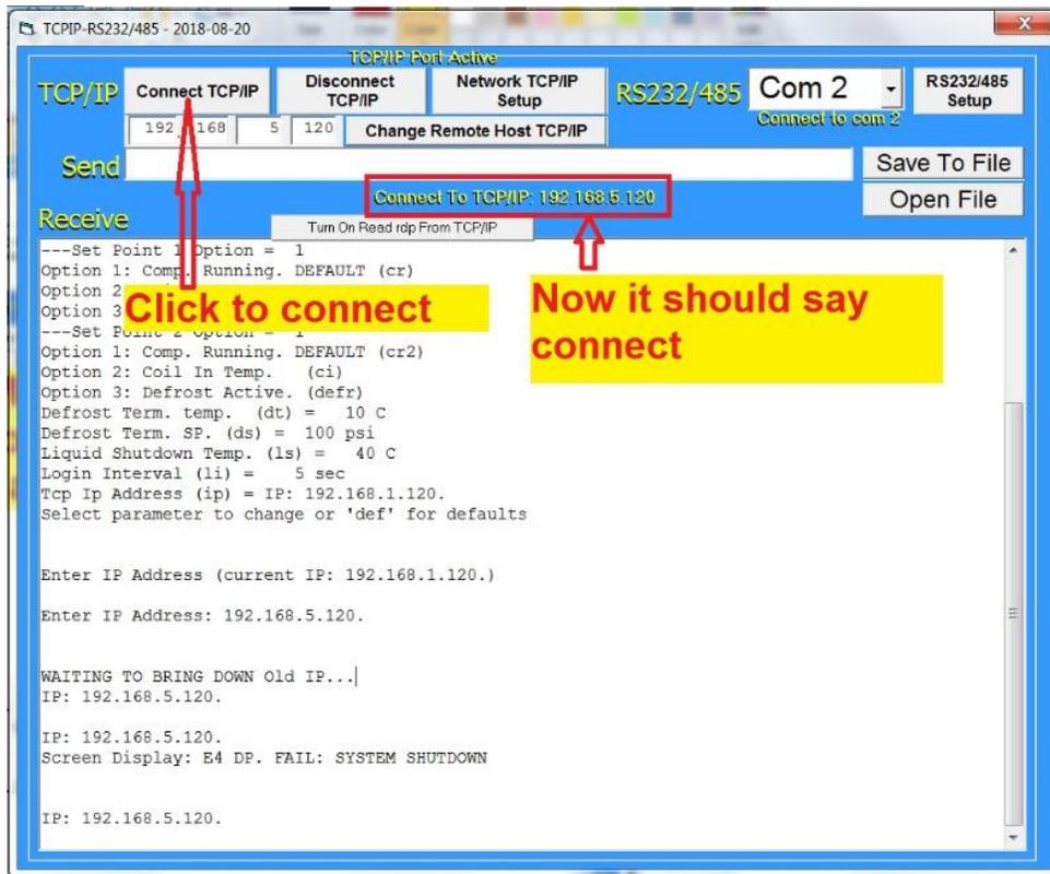
Figure 3-37, Connect to Remote Host
