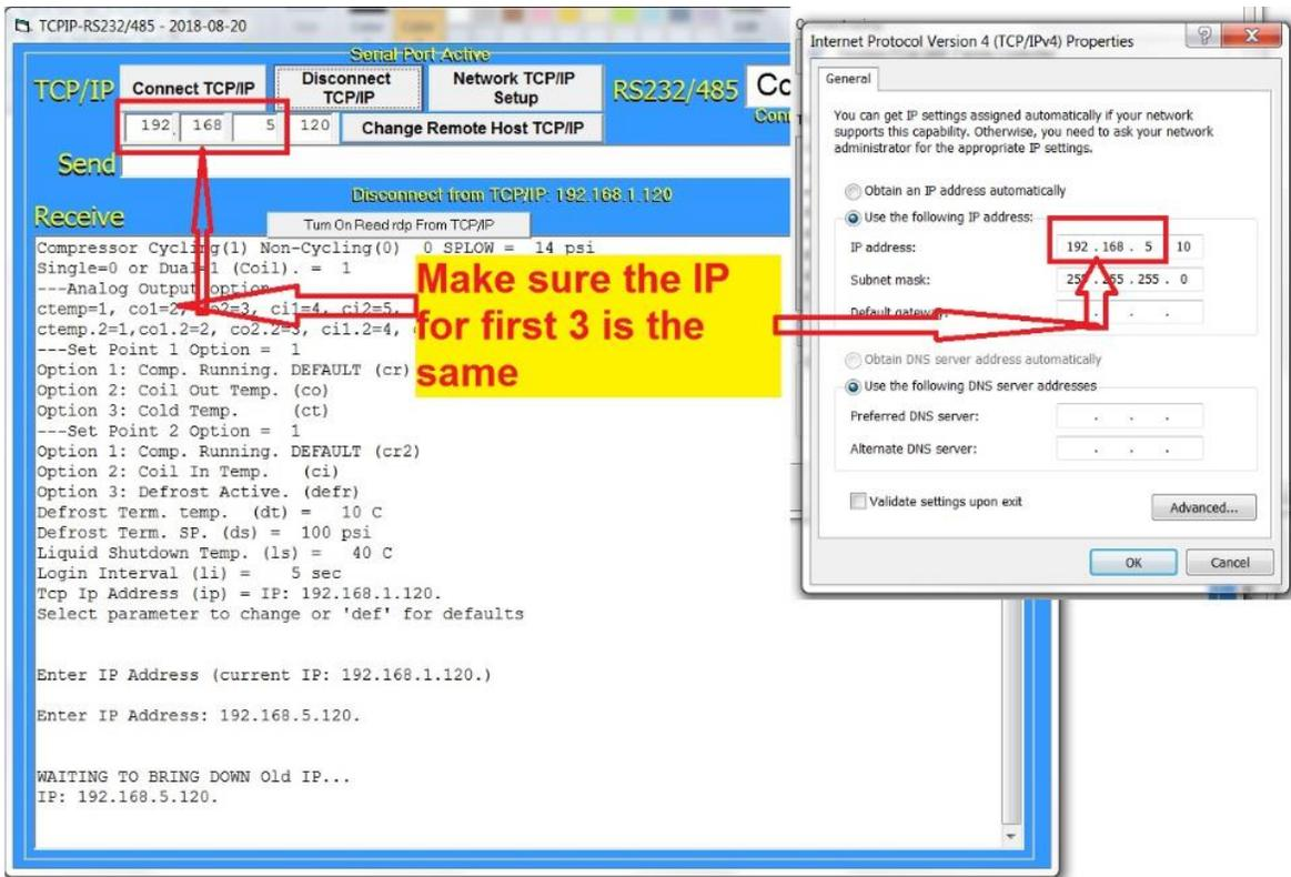
Figure 3-36, Check first three IP numbers
