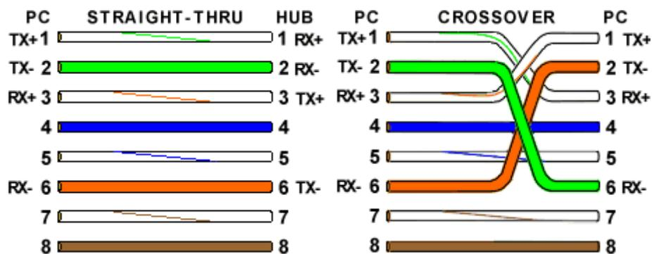
Figure 3-14, Ethernet cable (crossed)
