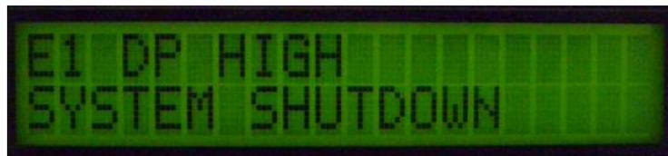
Figure 5-2, “E1” With Fault Shown as “DP HIGH”
