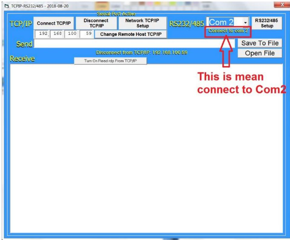
**Figure 3-24, Com Connection Shown**
