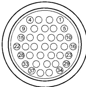
**Figure 3-13, 37-Way Amphenol™ Connector, Front view**
