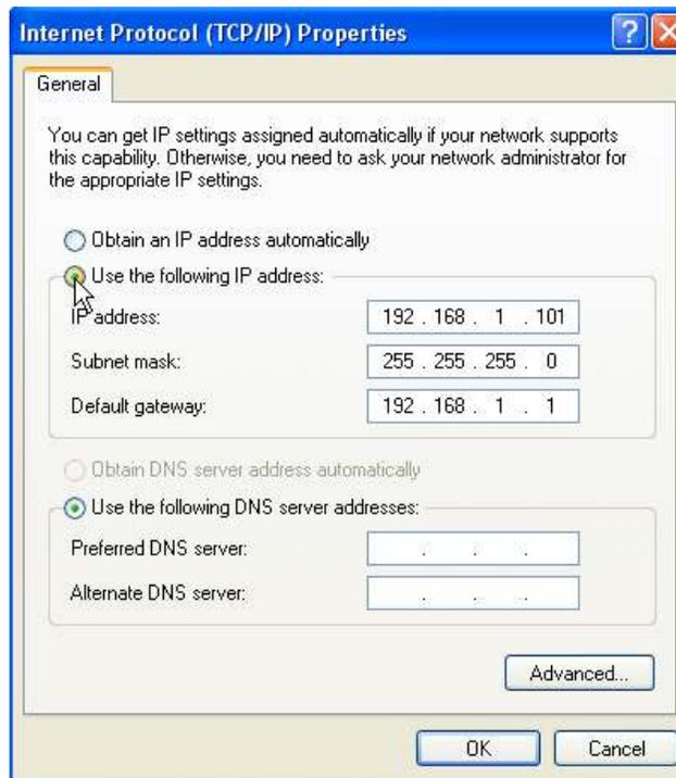
Figure 3-18, Set up for TCP/IP
