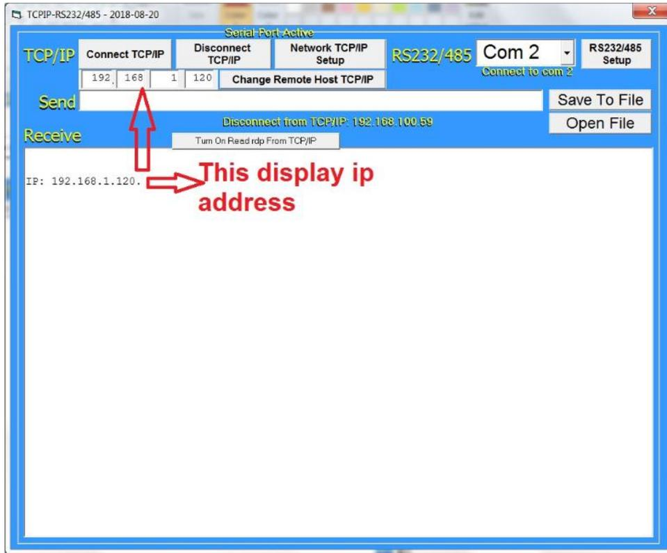
Figure 3-26 Display IP Address
