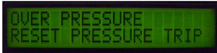
Figure 5-1, “OVER PRESSURE” Alarm Message
