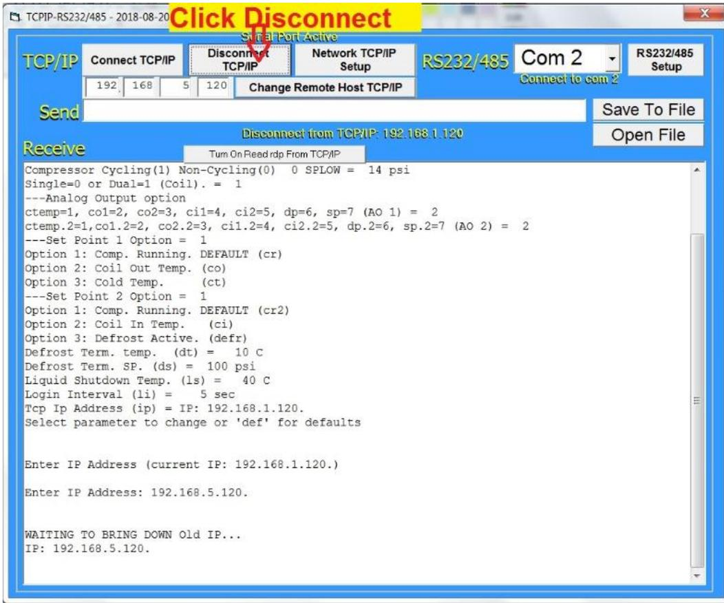
Figure 3-35, Disconnect TCP/IP Again
