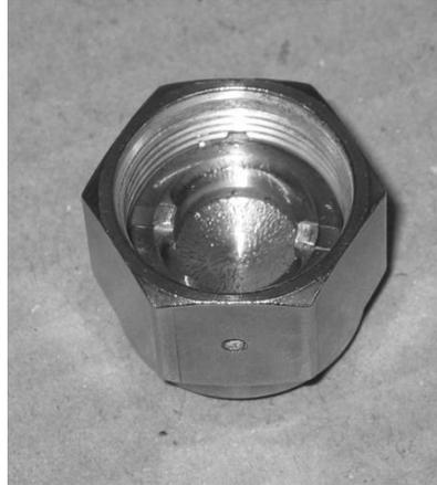
Figure 3-10, Metal O-ring Removal Tool
