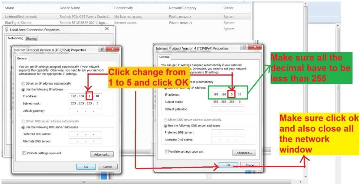
Figure 3-34, Change Remote Host IP address
