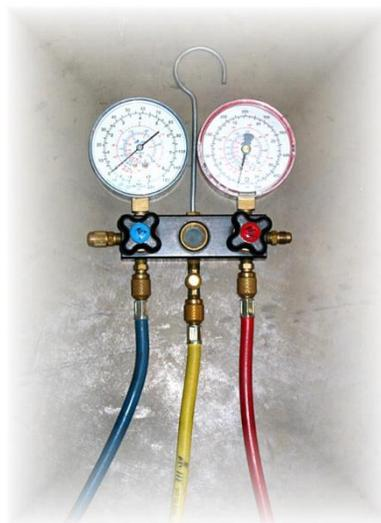
**Figure 3-8, Refrigerant Manifold**
