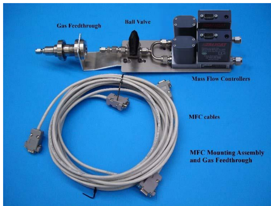
Figure 3-4, MFC Assembly
