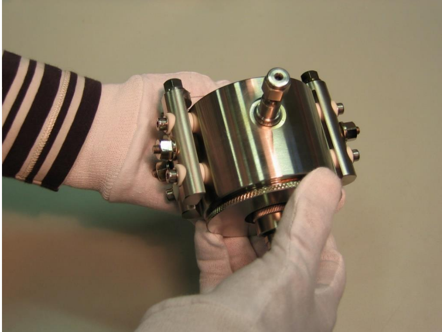
Figure 7-3, Unscrewing the knurled assembly nut
