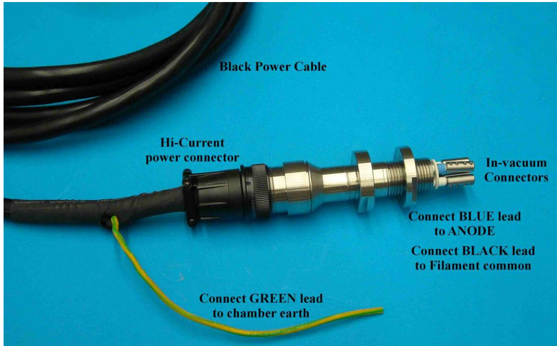
Figure 3-8, Electrical Feedthrough
