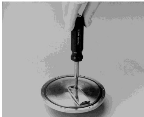
Photo 5 Fastening the Water Duct
