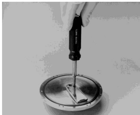
Photo 6 Fastening the Water Duct
