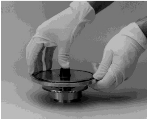
Photo 3 Inserting the Crucible Base
