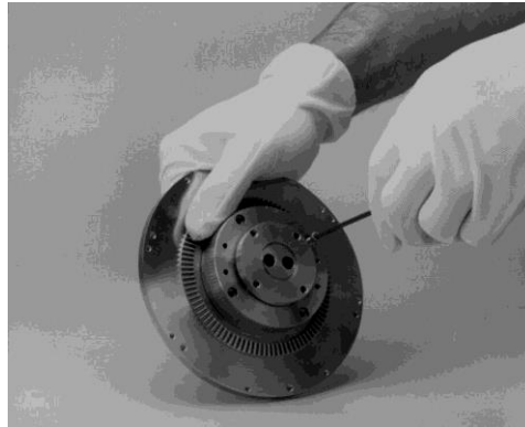
Photo 4 Fastening the Crucible Base
