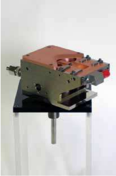
Photo 4 Place source feedthru through base plate
