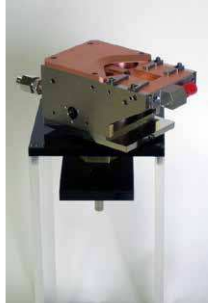
Photo 6 Mount Motor Clamp with three screws
