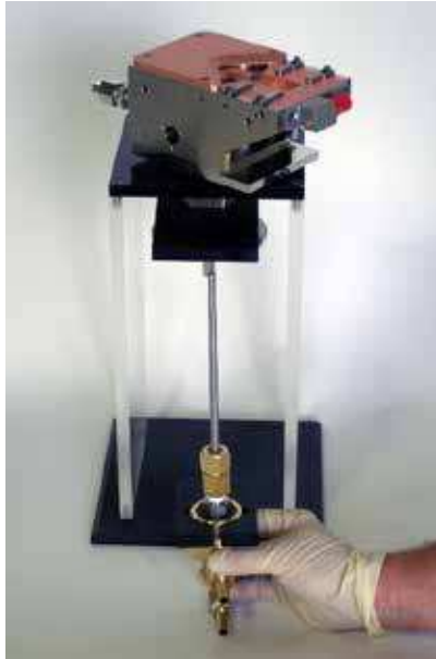
Photo 8 Install Water Union
