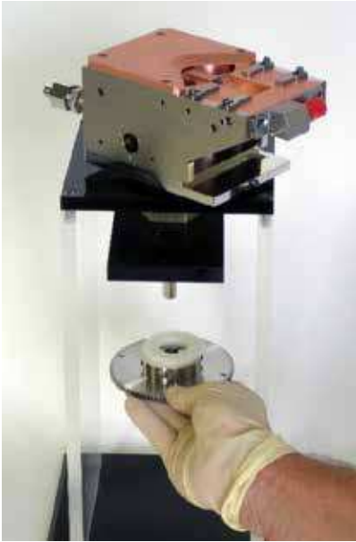
Photo 7 Place Motor Clamp Washers and Motor Clamp and Gear on shaft. Tighten Motor Clamp on Shaft, then tighten screws on Gear.
