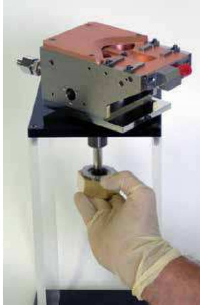
Photo 5 Install Feedthru Nut and Washer
