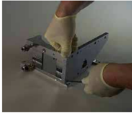
Photo 3 Fastening Magnet Arm
