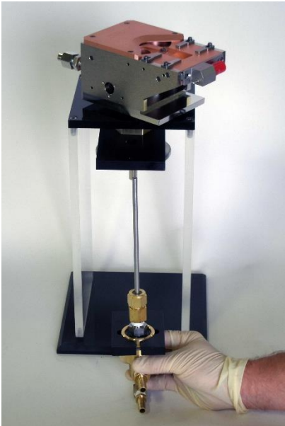
Photo 8 Install Water Union
