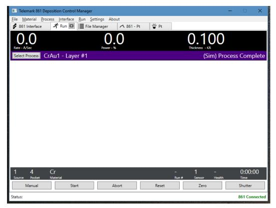
Press the "Select Process" button to bring up the Process/Film list. Select a Process or Film and press OK. All the layers will be loaded on the screen with the Layer number, Material, and Thickness Target.
