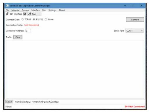
Numbers will appear on the screen. When finished it will report at the bottom the connection state and the Status. It should say "Finished downloading process list from 861" if not it will say "Unable to communicate with 861."
