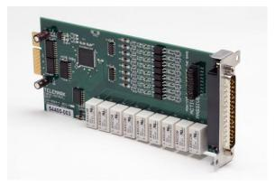
Figure 3-15, 37-Pin Input/Output Card
