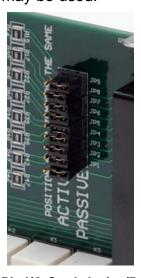
Figure 3-16, 37-Pin I/O Card, Active/Passive Jumpers
