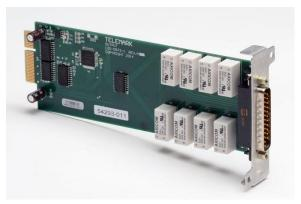
Figure 3-13, 25-Pin Output Card
