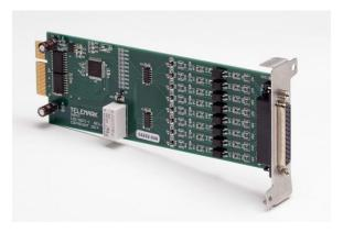
Figure 3-10, 25 Pin Input Card
