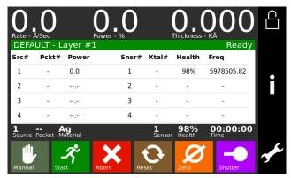
Figure 6-10, Source/Sensor Status screen
