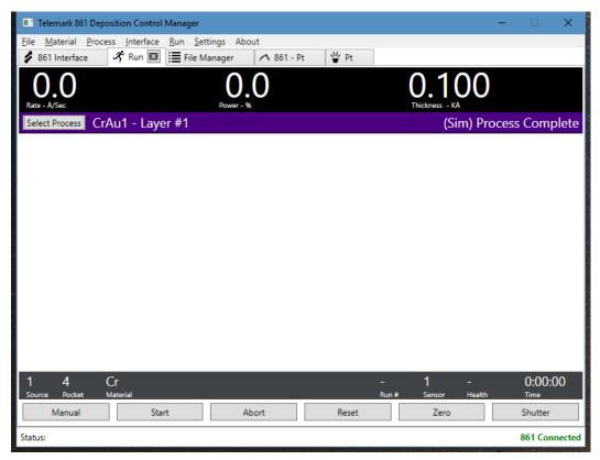
Press the "Select Process" button to bring up the Process/Film list. Select a Process or Film and press OK. All the layers will be loaded on the screen with the Layer number, Material, and Thickness Target.
