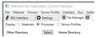
The file manager has three columns of Process or Material locations. The first column usually used for saving files on a computer hard disk. The Select button is used to change the location. The first column is not shown if not directory is selected.
