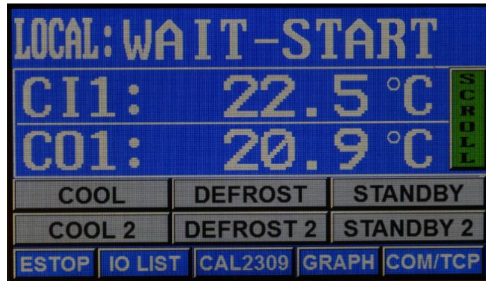
Figure 4-3, Coil In, Coil Out, Circuit One Display
