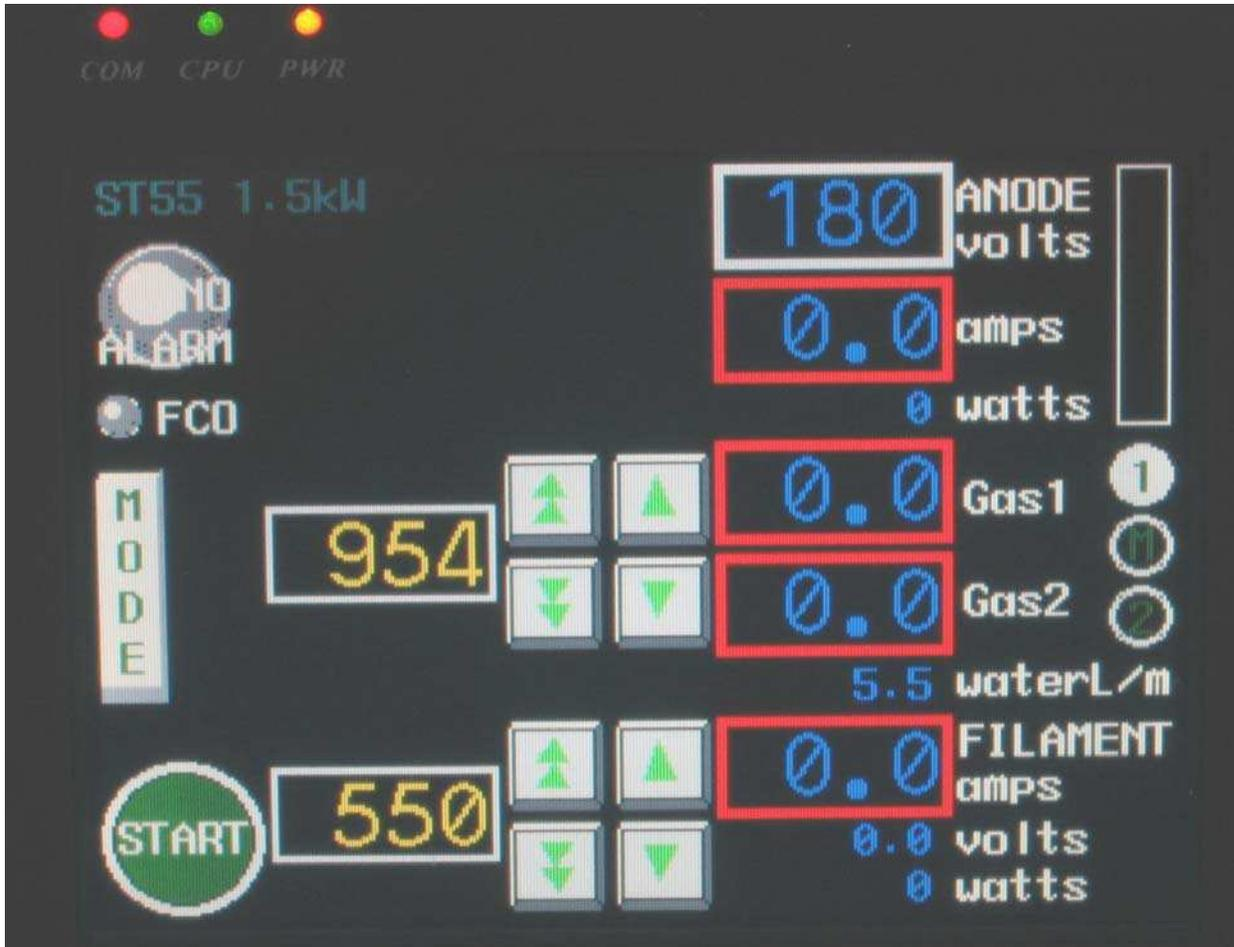
Figure above shows the main screen. This screen provides all functions to operate the Ion Beam System in the normal continuous mode.
