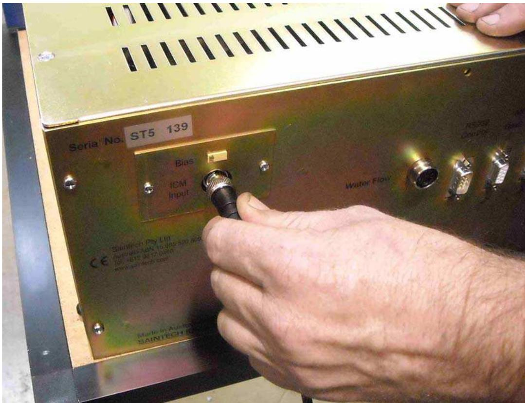
When the power supply is powered on the next time, it will recognize the installation automatically. The bias voltage can be adjusted over the full range by adjusting the small potentiometer located adjacent to the BNC connector on the rear panel.
