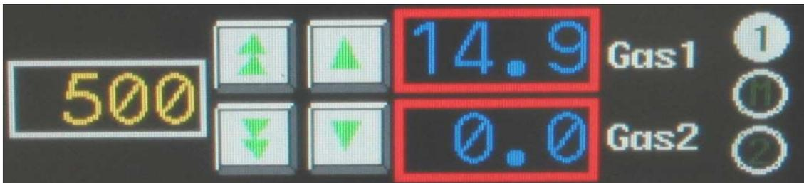
To use Gas 2 (argon) simply touch the Gas 2  button. Gas flow adjustments will now relate only to argon gas. Note that, if the source gas is changed (Gas 2 → Gas 1), the last used Gas 1 setting will now be selected.
