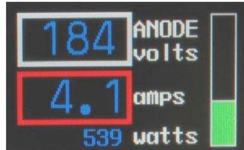
the green bar graph to the right of the screen. As the power level increases the green ‘bar’ rises in the window. In the event that the maximum allowable power is achieved, the green display changes to red and the “amps” flashes in red. Any attempt to further increase beam power by increasing gas flow will be unsuccessful.
