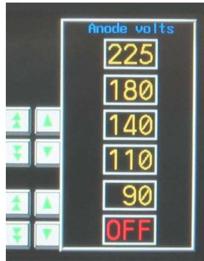
Note that the voltage displayed while the power supply is in standby, is the ‘nominal’ anode voltage. The actual and instantaneous anode voltage is shown once the power is ON. The voltage shown will then be the peak anode voltage and will generally be slightly higher than the nominal voltage when no beam current is produced. It is normal for the anode voltage to reduce as beam current increases and may be seen to be lower than the nominal voltage at high power levels.
