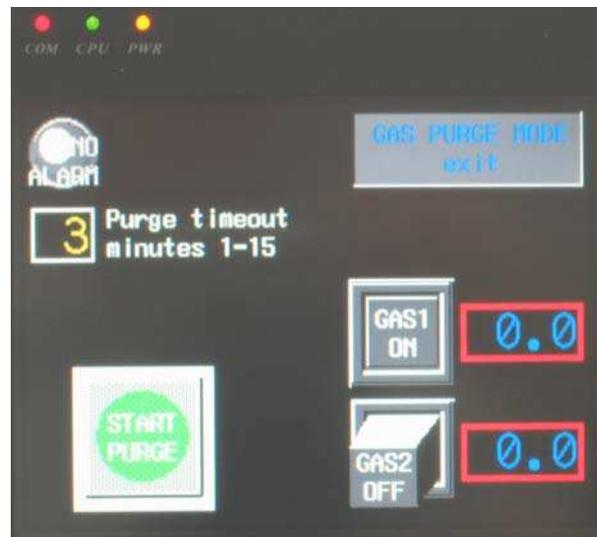
timeout for about 1 minute longer. In the event that a flow of 1 – 2% cannot be reached the possibility of a leak should be investigated.
