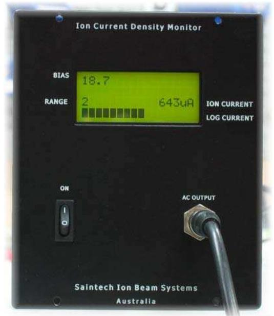
The digital data from the ICM is auto-ranging and covers the range from 1 microamp to 2 milliamps. The data displayed is the RMS ion current as measured in the **ICM** sensor.
