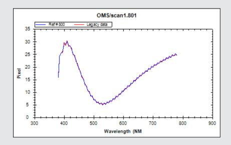
A spectral match can be determined by an evaluation of the lowest or best possible match. The following graphic describes the fit for the above match.
